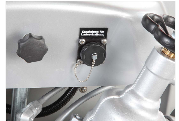
■ BEOS ELECTRICAL OUTLET 1146206 Three-pole screw-type outlet for charge maintenance of the UP4 for the BEOS-vehicle installation kit.
